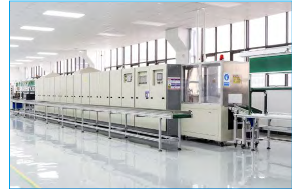
Tunnel Furnace Brazing
